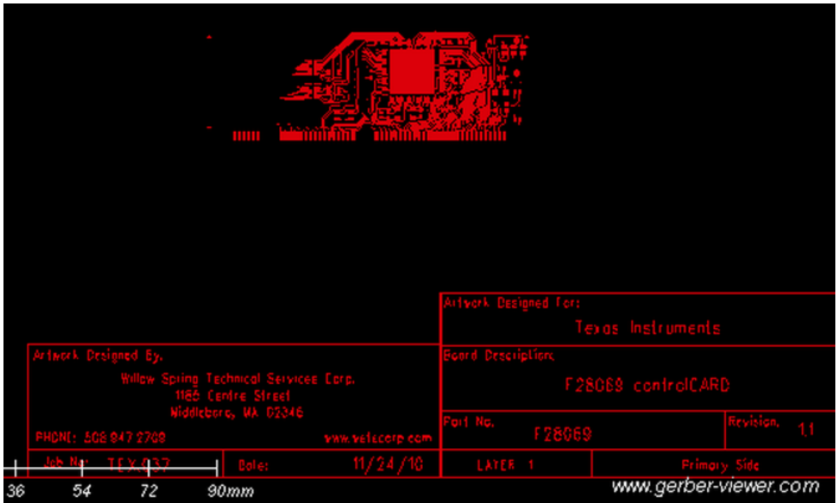
Figure F6.2B – Gerber Photoplot
